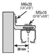
Conector Muro Ancho
