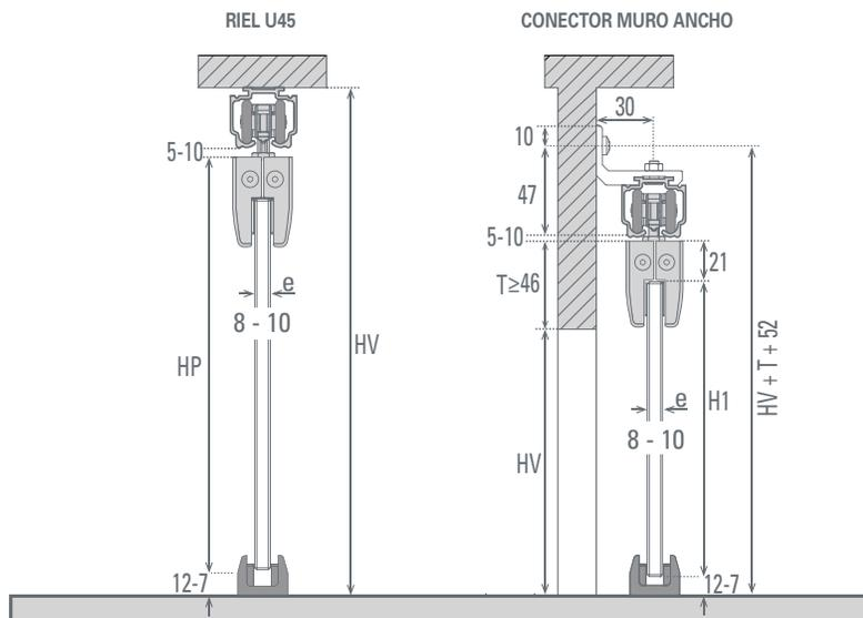
$$\begin{aligned} HP &= HV - 48 \\ H1 &= HV - 69 \end{aligned}$$
